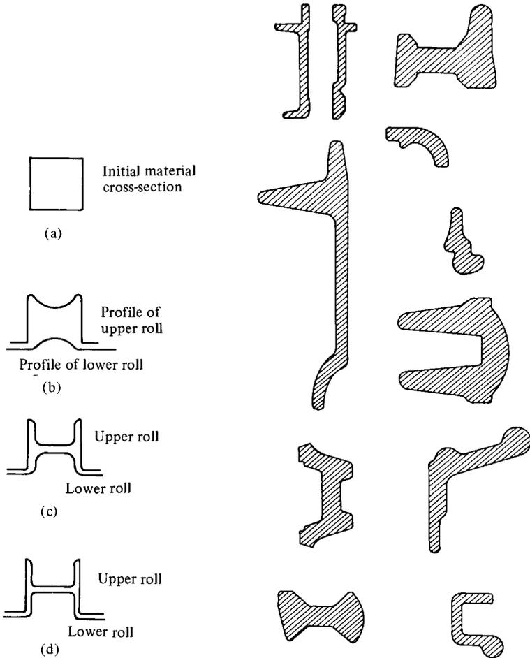
**Figure 1.5** (a) The type of rolling sequence used for a structural beam section (b), (c), (d) Examples of rolled sections
