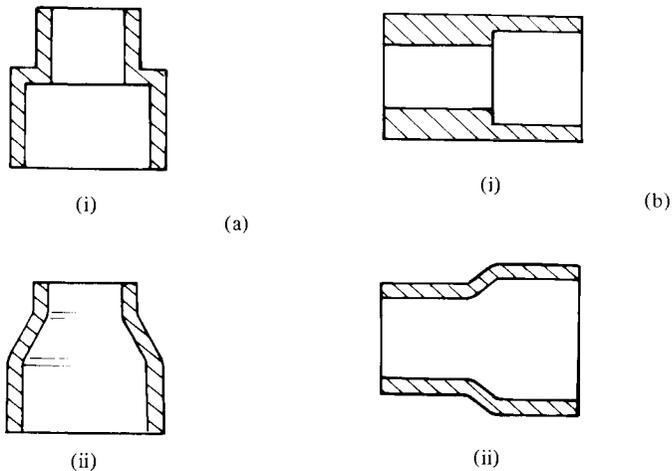
**Figure 1.4** (a) The need for no sharp corners in casting means (ii) is preferred to (i) (b) The need for uniform thickness sections in casting means (ii) is preferred to (i)
