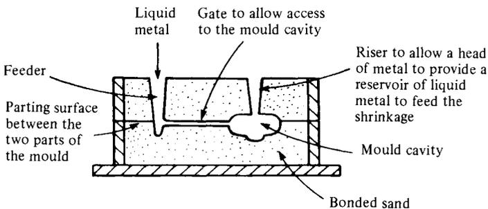
**Figure 1.2** Sand casting
