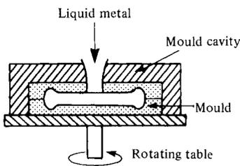
**Figure 1.3** Centrifugal casting
