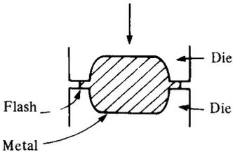
**Figure 1.6** Closed die forging
